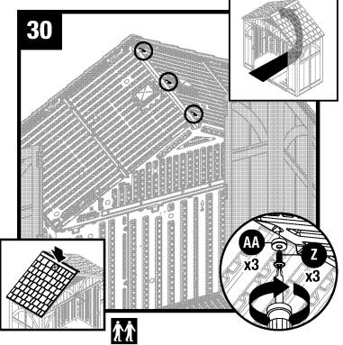
Push down the roof from outside. From inside shed, secure roof panels together along ridge of roof using three rubber washers (AA) and three sealing screws (Z).
