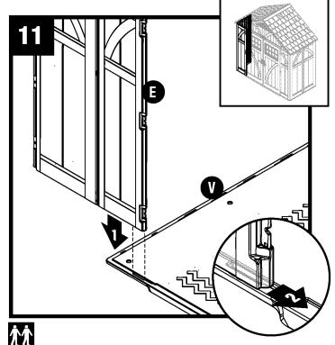
Align tab on bottom of left front corner (E) with slot on left floor (V). Lower panel into slot and lock in place by sliding panel toward door opening.
