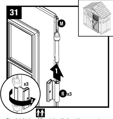
Stand right door (M) upright with three hinge mounts facing right. Slide one metal door hinge (R) up onto each hinge mount. Rotate door hinges to outside of door.
