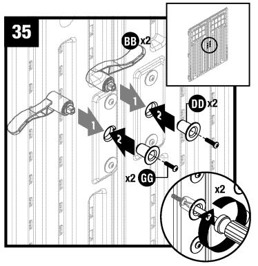
From the outside of doors, insert door handles (BB) through handle plate holes. On inside of doors, place spacers (DD) on each door handle, and secure each with one pan head screw (GG).
