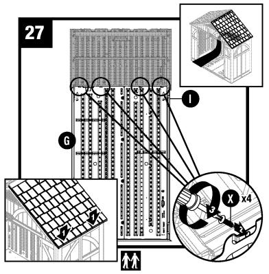
Pull down each lower corner of roof from outside. From inside shed, attach tabs on right front corner (I) & rear corner (G) to roof panel with four screws (X).
