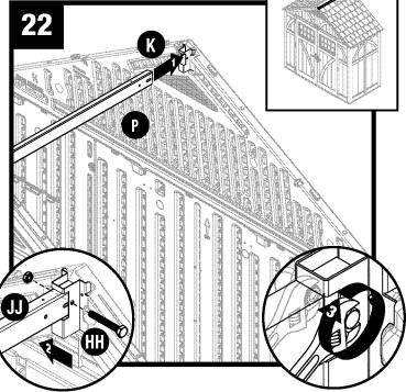
Raise ridge beam (P) up and into rear header (K). Secure with one bolt (HH) and one nut (JJ). DO NOT tighten.
