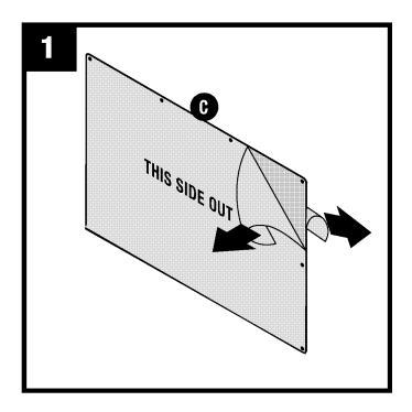
Peel film from both sides of window (C). Remove protective film from door edges.
