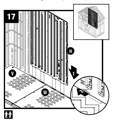
Align tabs on bottom of back panel (H) with slots along floor (V) & (W). Lower panel into slots and lock in place by sliding panel toward rear corner.
