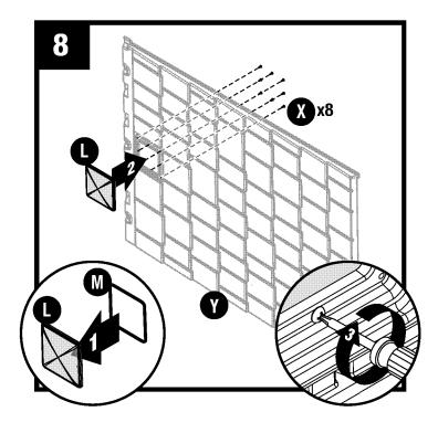
Place skylight gasket (M) into skylight (L). Place skylight (L) onto right roof panel (Y). Secure from underside with eight screws (X). Make sure rib on plastic parts is seated fully against gasket on skylight.
