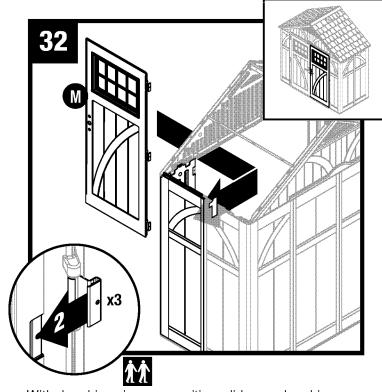
With door hinge in open position, slide one door hinge over each hinge receptacle on inside of right front corner.
