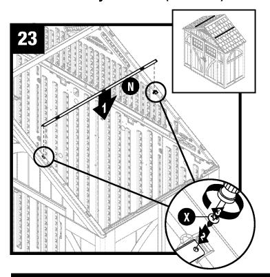
Attach roof support bracket (N) to front and rear headers. Secure with two screws (X).
