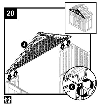
Place front header (J) over door opening and fit four protruding support legs into pockets molded in front corners. Secure front header using two screws (X).
