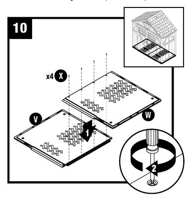
Push left floor (V) and right floor (W) panels together and secure with four screws (X).
