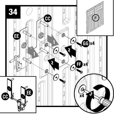
Insert screw stems, on left and right handle plates (EE) and (CC), through the holes in doors. While holding plates in place on exterior of door, secure each with two washers (FF) and two pan head screws (GG).
