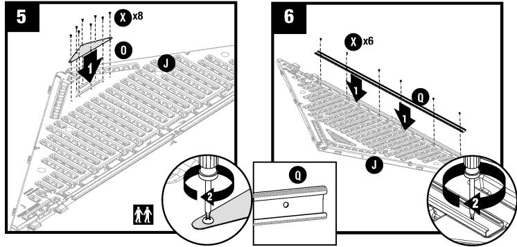
Lay front header (J) on ground with lettering side facing up. Place fiberglass vent screen (O) into rear opening in front header (J). Secure with eight screws (X).
