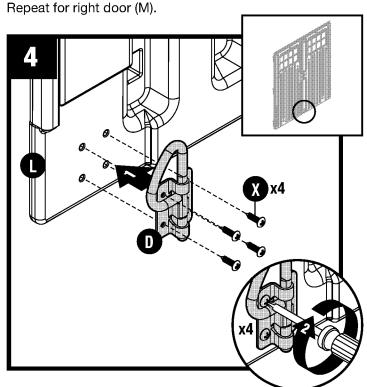
At bottom interior side of left door (L), attach D-ring slide bolt (D) with four screws (X).
