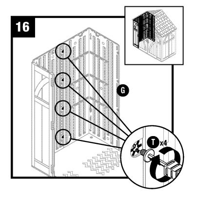
Secure rear corner panel (G) with four easy bolts (T), working from floor to roof. **DO NOT** use torque wrench. Use easy bolt easy driver (U) and hand tighten. Easy bolt head will be flush when fully seated. **DO NOT** over tighten easy bolts.
