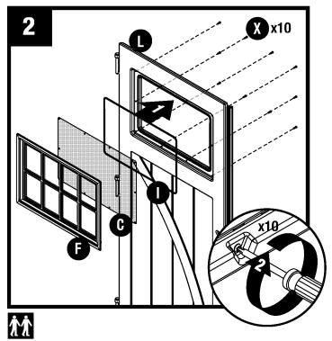
Place gasket (I), window (C), and frame (F) into door channel. Secure with ten screws (X), starting at corners. **DO NOT** over tighten screws. Repeat for remaining door.
