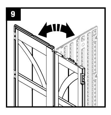
**Critical:** When installing corners, flex corner hinges back and forth several times. This will help provide a square corner and ensure proper fit of remaining panels.
