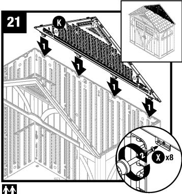
Place rear header (K) over back walls and fit four protruding support legs into pockets molded in back walls. Secure rear header using eight screws (X).
