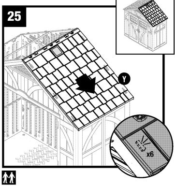
Slide right roof (Y) down towards the outside of shed. You will hear a "snap" when engaged.
