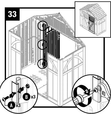
Secure each metal hinge plate with one screw (A) and one nut (B). Repeat Steps 31-33 for left door (L).
