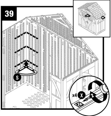
Attach shelf (S) in desired location with four screws (X) Repeat for remaining shelf (S).
