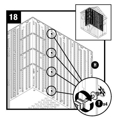
Secure back panel (H) with four easy bolts (T), working from floor to roof. **DO NOT** use torque wrench. Use easy bolt easy driver (U) and hand tighten. Easy bolt head will be flush when fully seated. **DO NOT** over tighten easy bolts.
