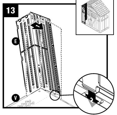
Tip left front corner (E) back to vertical position and align lower tabs on right side with slots in floor (V).
