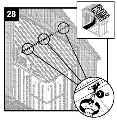
Secure roof support bracket (N) to roof using three screws (X).
