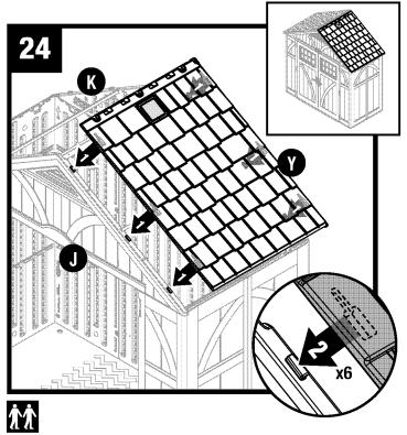
Lay right roof (Y) directly over three tabs on right side of front header (J) and three tabs on right side of rear header (K). With right roof slots seated over/on header tabs, check alignment in all six spots.
