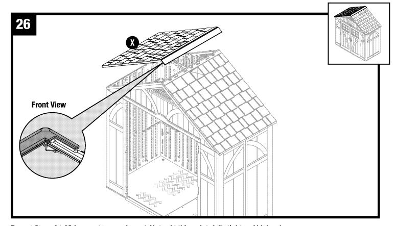
Repeat Steps 24-25 for remaining roof panel. Note: At this point, fully tighten ALL hardware.
