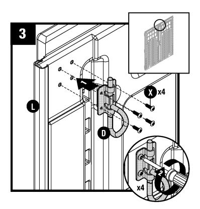
At top interior side of left door (L), attach D-ring slide bolt (D) with four screws (X).
